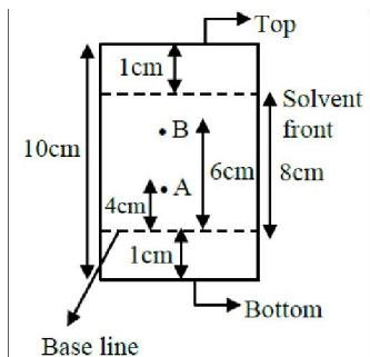
$$(R_f)_A = \frac{4}{8} \quad (R_f)_B = \frac{6}{8}$$
