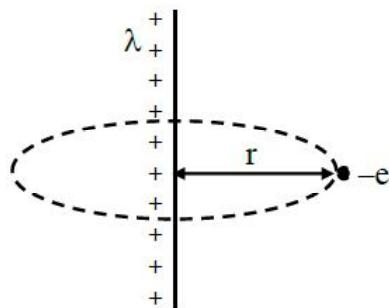
Electric field  $E$  at a distance  $r$  due to infinite long
