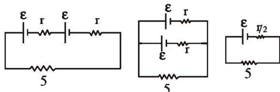
$$i = \frac{2\epsilon}{5 + 2r} \quad \dots\dots(1) \quad i = \frac{\epsilon}{\frac{r}{2} + 5} \quad \dots\dots(2)$$
