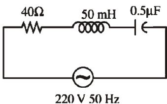
$X_L$  is not equal to  $X_C$ . So rms current in (b) can never be larger than (a).
