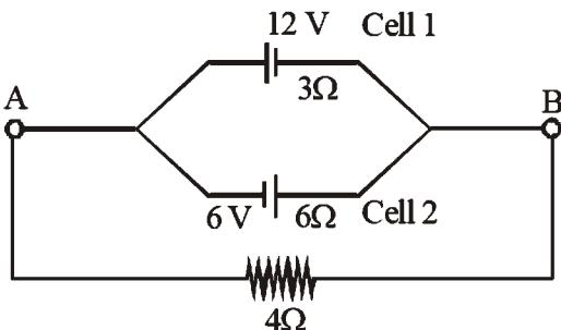
$$E_{\text{eq}} = \frac{\frac{12}{3} - \frac{6}{6}}{\frac{1}{3} + \frac{1}{6}} = \frac{1}{1} = 1 \text{ V}$$
