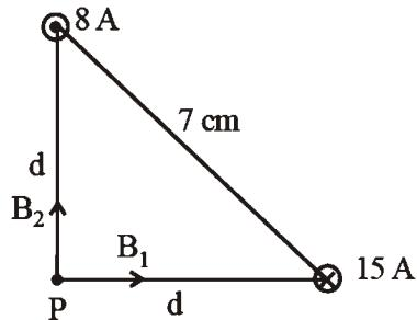
Magnetic fields due to both wires will be perpendicular to each other.
