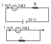
(A) for voltmeter  $R \approx 50 \text{ k}\Omega$  (B) for ammeter  $\approx 0.2 \Omega$
