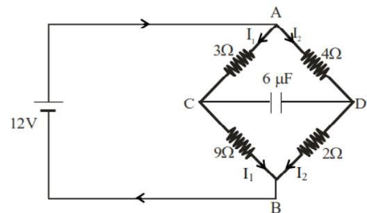
$$V_A - V_C = 3I_1 = 3V \quad \dots(1)$$
