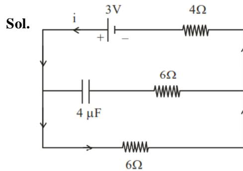
No current will flow in capacitor in steady state, current flowing in the circuit in steady state
