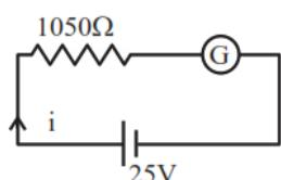
$$i = \frac{25}{1050 + R_G} \quad \dots\dots(ii)$$
