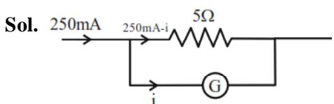
$$\frac{250\text{mA} \times 5}{5 + R_G} = i \quad \dots\dots(i)$$
