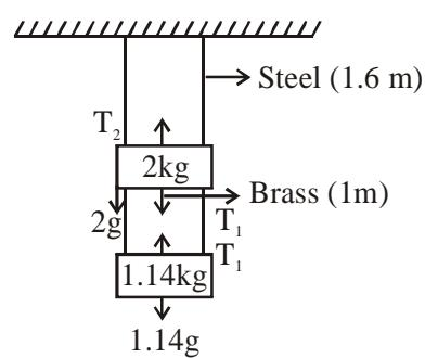
Elongation in steel wire  $\Delta L = \frac{T_2 L}{A y}$
