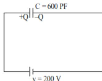
$$Q = CV = 600 \times 10^{-12} \times 200 = 12 \times 10^{-8} \text{ C}$$
