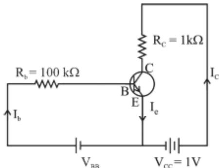
Considering the transistor in saturation mode
