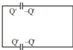
Charge will be equally distributed on identical capacitor
