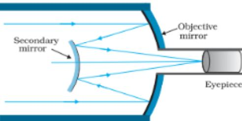
It has advantage of a large focal length in a short telescope
